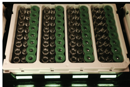
Fig. 7. A, DG32 Cartridge holders on the AutoDG deck in the “Load” state, indicated by yellow lights; B, green lights indicate the DG32 Cartridge has been correctly loaded and is ready.
