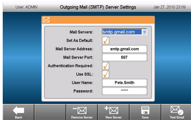
Figure 10. Gmail server is selected, user name and password have been entered, and server has been selected as the default server.
