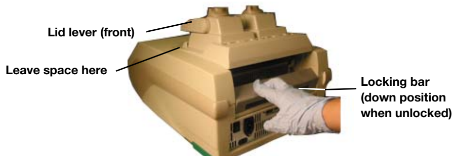
Figure 4. Inserting the reaction module into the bay.
