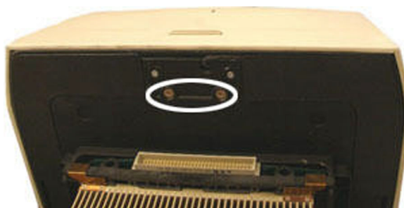
Figure 108. Remove these screws to unlock the optical module.
