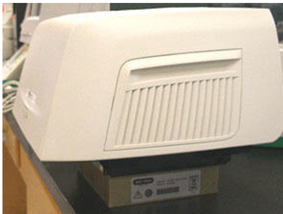
Figure 107. Setting up the Optical Module to remove the locking plate.
