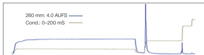
E. Bioreactor = 50 L; Column = 600 ml; Flow rate = 200 ml/min
