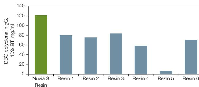
**Fig. 3B. Binding of polyclonal human IgG by Nuvia S Resin.** Comparison of Nuvia S and other commercially available CEX resins. Column size, 0.7 x 5.5 cm. The sample was loaded onto the column in 40 mM sodium acetate, pH 5.0 + 30 mM sodium chloride, washed, and then eluted with 40 mM sodium acetate, pH 5.0 + 1 M sodium chloride. DBC, dynamic binding capacity; BT, breakthrough.
