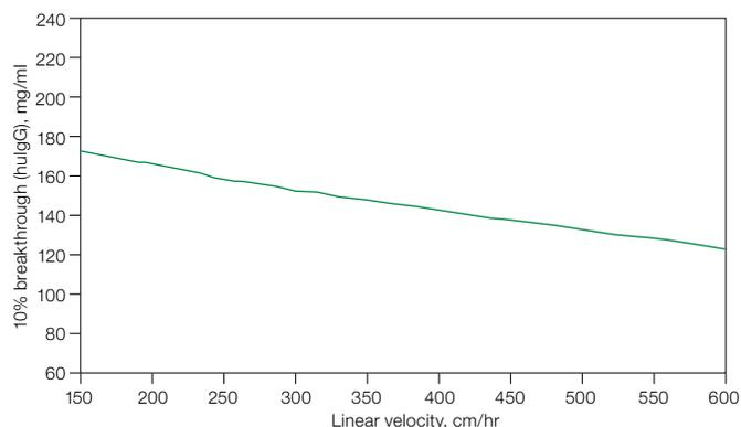
**Fig. 3A. Binding of hulG by Nuvia S Resin at varying linear velocities.** Column size, 1.1 x 20 cm.
