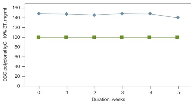
**Fig. 4. Stability of Nuvia S.** Results from an accelerated storage study (in 1 N NaOH) show no loss in dynamic binding capacity and recovery. hIgG binding capacity, 10% breakthrough (◆); recovery (%) (■); BT, breakthrough; DBC, dynamic binding capacity.
