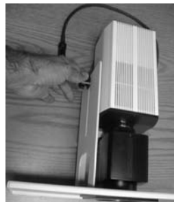
Tighten the black knob to secure the camera to the bracket assembly
