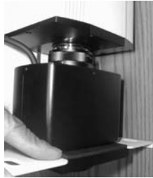
i. The lens body should be completely flush against the rubber gasket
