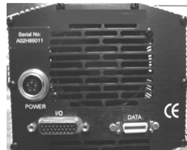
Controller Cable Connector labeled Data
