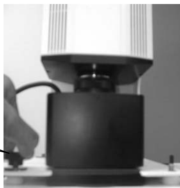
Secure the bracket to the hood at four studs using the four knobs and washers.
