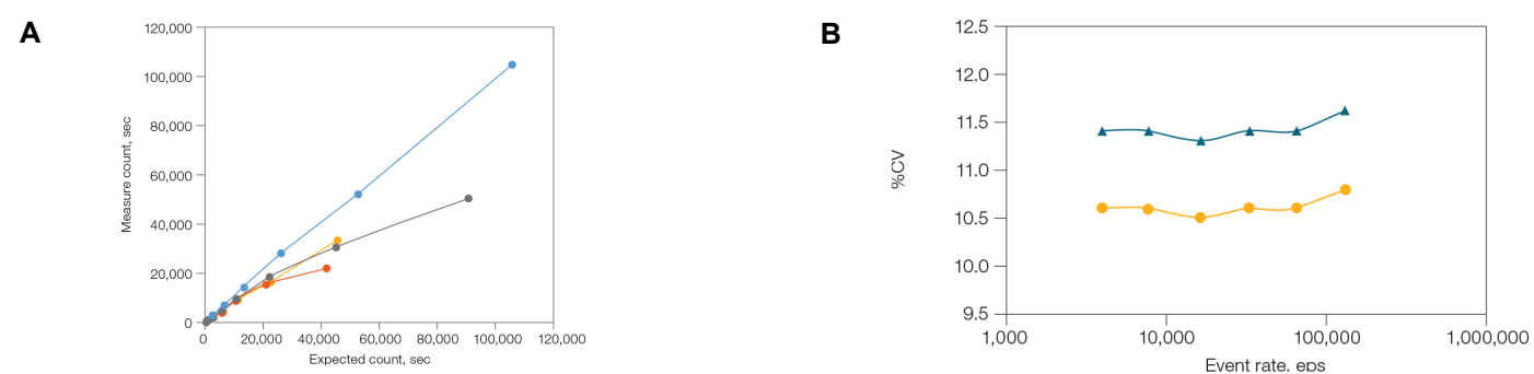
Fig. 1. Speed and signal stability. A, the ZE5 Cell Analyzer outperforms other systems at higher acquisition speeds because it continues to acquire data in the 100,000 events per second range, whereas other systems drop off around 20,000 events per second. Dragon Green Beads (Bangs Laboratories, Inc.) were used in a serial dilution to determine when the observed acquisition rate falls off the theoretical limit. ZE5 Cell Analyzer (—); cytometer 1 (—); cytometer 2 (—); cytometer 3 (—). B, beads were read at increasing events-per-second rates, and singlet beads were gated using pulse geometry gating. The percentage CV of side scatter (SSC) and fluorescein isothiocyanate (FITC) was plotted over approximately 4,000–129,000 eps. The mean and standard deviation (SD) of CVs over this range were FITC-A (●): mean = 10.6, SD = 0.063; SSC-A (▲), mean = 11.4, SD = 0.063.
