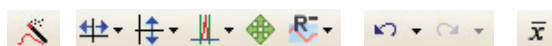
Fig. 8. Quick navigation to processing controls. From left to right: 3-point auto processing; individual processing keys for manual or automated X and Y alignment, spike removal, manual sensorgram movement, and referencing; undo and redo commands; report point generation commands.
