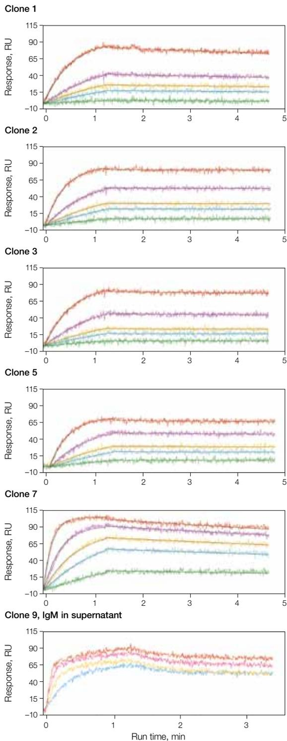
**Fig. 3. Rapid screening of unpurified hybridoma supernatants to obtain ranking data.** Shown are sensorgrams of six hybridoma clone supernatants, five exhibiting conventional 1:1 Langmuir binding, and a sixth displaying complex binding kinetics due to the presence of IgM in its supernatant. Black lines represent global fits of the sensorgrams to the 1:1 Langmuir interaction model. See Table 1 for the kinetic rate constants of these data.
