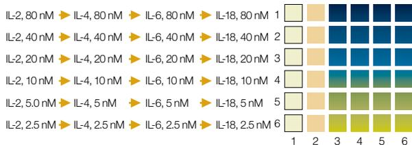
**Fig. 8. Multiple antibody-antigen specificity analysis.** Representative protocol for analysis of multiple purified antibodies with multiple antigens. Use of hybridoma supernatants requires immobilization of a capture anti-mouse antibody to the chip surface. Each 6 x 6 specificity analysis is followed by sensor chip regeneration.
