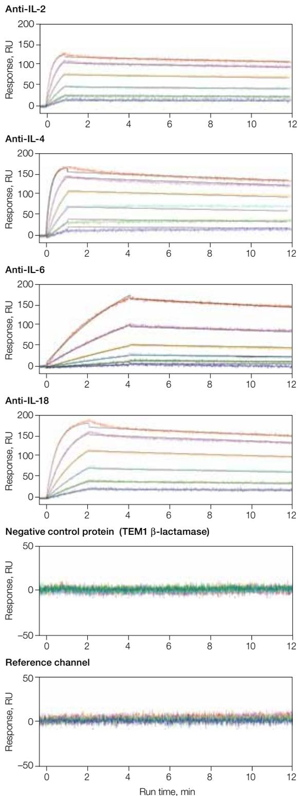
**Fig. 9. Four representative sets of six sensorgrams showing global fits to each specific antibody-antigen interaction, with negative control and reference channel plots.** For details, see Bronner et al. (2006).
