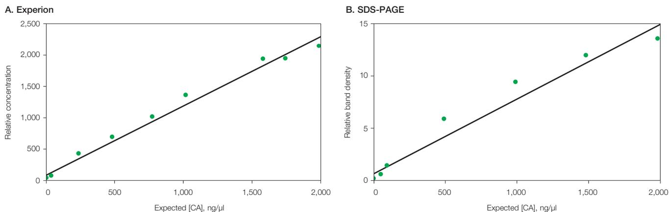
**Fig. 2. Comparison of linear dynamic range of protein separation.** Samples of CA at the concentrations indicated were separated with the Experion Pro260 analysis kit or by SDS-PAGE. The relative concentration or band density obtained from the Pro260 (A) and SDS-PAGE (B) analysis was plotted as a function of concentration. Representative graphs are shown. The  $r^2$  values for a linear fit of the data sets were 0.9887 (A) and 0.9626 (B).
