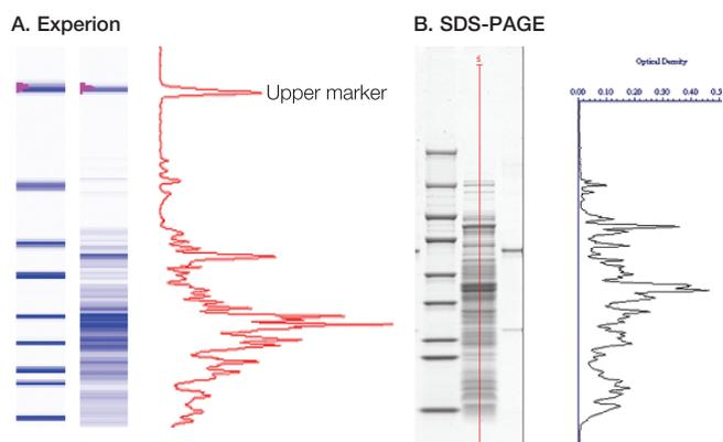
**Fig. 3. Comparison of protein detection using an *E. coli* lysate.** **A**, simulated gel view (left) and electropherogram (right) of separation with the Experion Pro260 analysis kit; the peak generated by the upper marker is indicated; **B**, gel image (left) and Quantity One software analysis (right) of separation by SDS-PAGE. A comparable number of peaks were identified using both separation methods.
