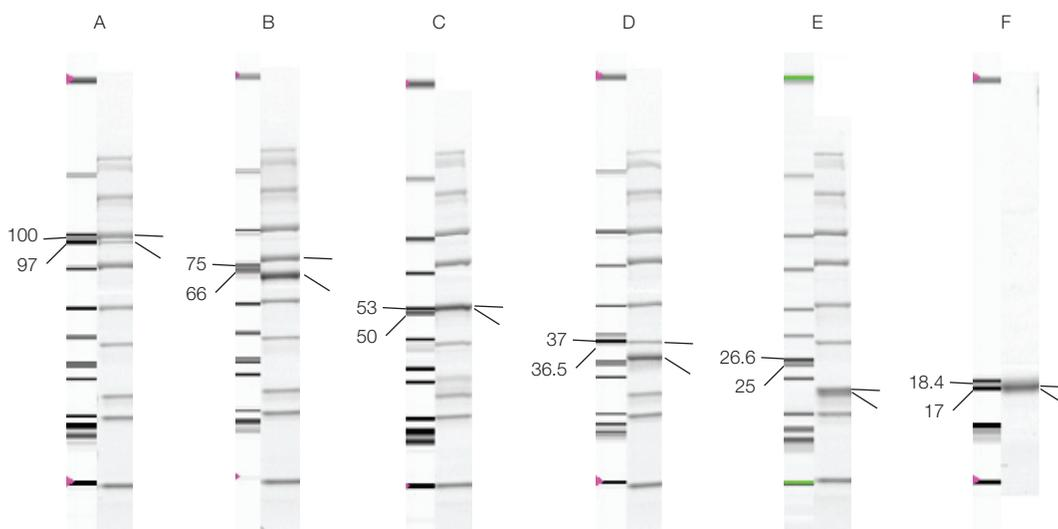
**Fig. 4. Comparison of separation of pairs of proteins with the Experion Pro260 analysis kit and SDS-PAGE.** For each protein pair listed in Table 4, the left panel shows the Experion simulated gel view, and the right panel, a scanned SDS-PAGE gel image.
