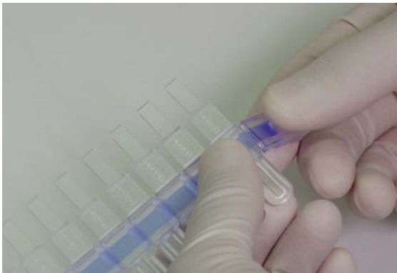
Fig. 2. Break and twist off one end of the plastic plug casing.
