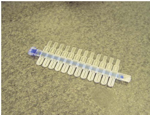
Fig. 1. Flat side of plastic casing with 12 Precision Plus Protein standard plugs, unstained.
