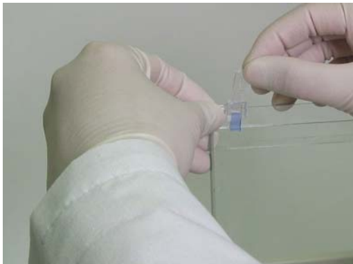
Fig. 7. Use the spatula to slide the plug outward and on to the top plate of your gel.
