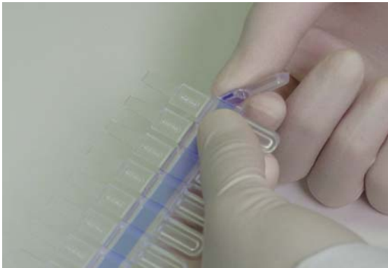
Fig. 4. Complete the break by twisting off the individual plastic plug casing.
