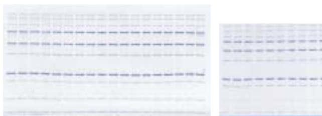
Criterion XT gels separate more samples in fewer runs. Precision Plus Protein standards separated on a 12% Criterion XT Bis-Tris 18-well gel with XT MOPS buffer (left) and on a competitor's 12% Bis-Tris 10-well mini gel (right).
