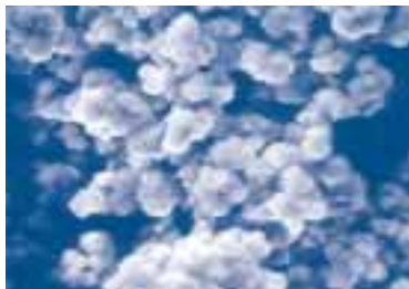
Fig. 1. The structure of the Continuous Bed matrix can be seen in this scanning electron micrograph (1.95k magnification). Note the fimbriated structure of the polymer nodules and the large channels between them.
