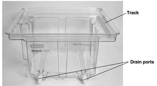
Fig. 2.3.1 D. Solution tank.
