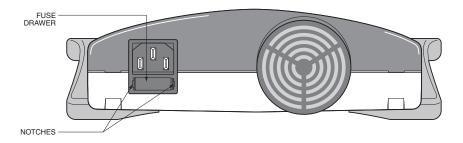
Fig. 7. Rear view Showing Fuse Drawer with Notches.
