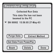
Select a data file from the drop-down **Run Data** list and then press **Beam** to transmit the data to a PC. The warning "This data file has not been beamed to the PC" is displayed for all data files that have not been transmitted to a PC. Note that the **Extract Method**, **Beam** and **Delete** buttons appear only if a run in the **Run Data** list has been selected.
