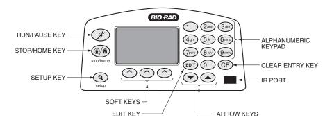
Fig. 4. Front Panel.
