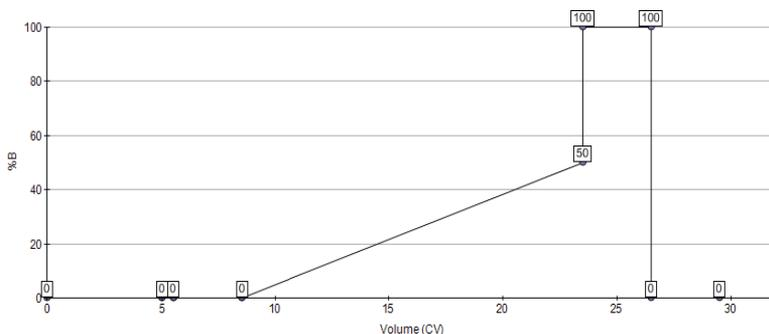
**Fig. 1. Schematic gradient for separation on an ENrich IEX column.** Volume, column volume.
