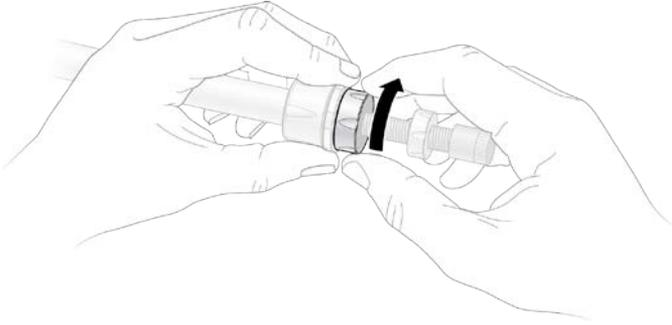
**Fig. 8.** Lower the adaptor by turning the adjusting nut clockwise.
