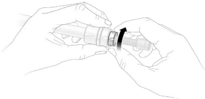
**Fig. 4. Loosen the lock nut by turning it clockwise.**
