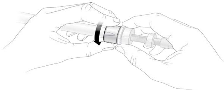
**Fig. 7. Reattach and hand-tighten the retainer.**
