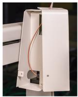
Connect the sample tube to the dispense head. Use the cutout in the back of the cover to insert a fittings tightener and tighten.
