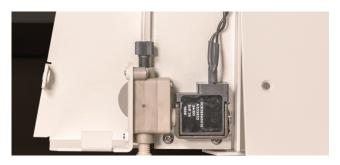
4 Route both tubes through the top of the dispense head cover by sliding them into the rubber grommet. Finally, close the dispense head cover and fasten with the screw.
