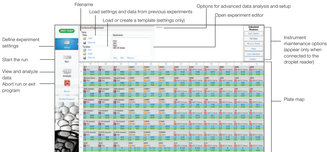
QuantaSoft software Setup interface. The plate map is a diagram of the wells in the 96-well plate and contains information about the type of analysis, sample, and assay represented by that well. After a run, it also contains concentration data.
