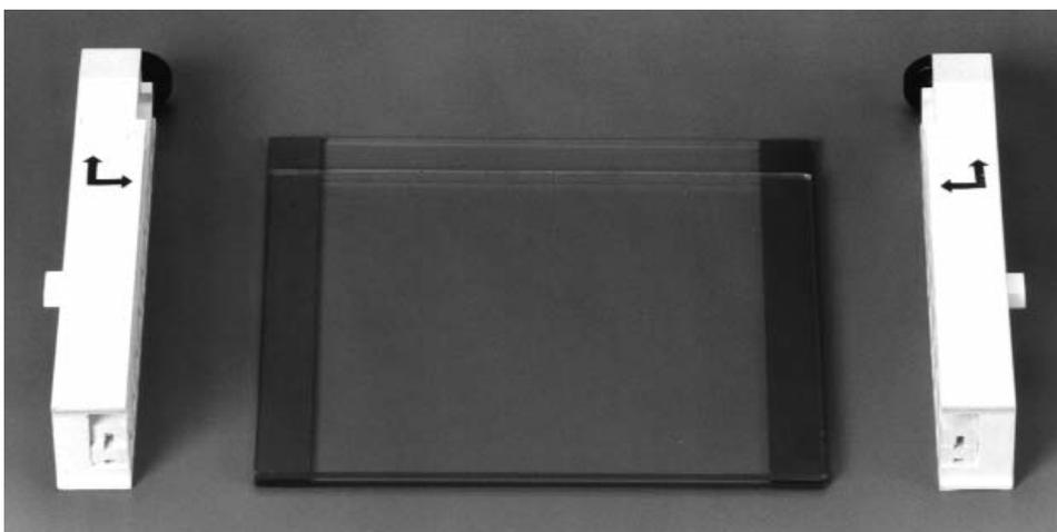
Fig. 4.24. Positioning glass plates, spacers, and clamps.
