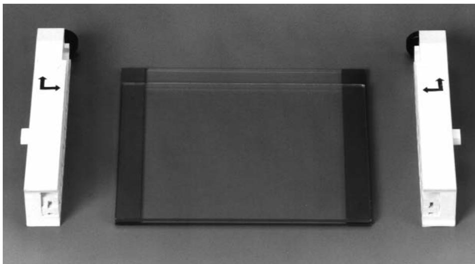
**Fig. 7.2. Positioning glass plates, spacers, and clamps.**
