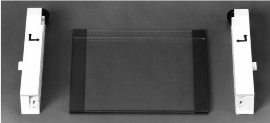
Fig. 6.3. Positioning glass plates, spacers, and clamps.
