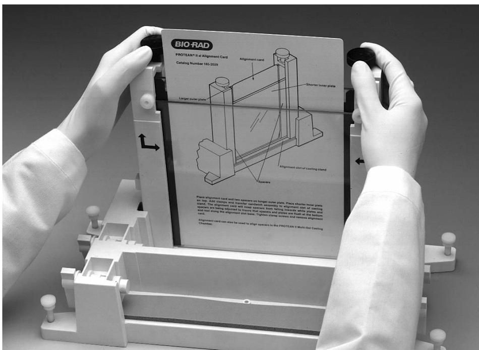
**Fig. 4.19. Aligning spacers in the sandwich assembly.**
