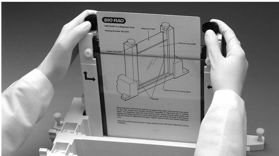
Fig. 4.12. Aligning spacers in the sandwich assembly.
