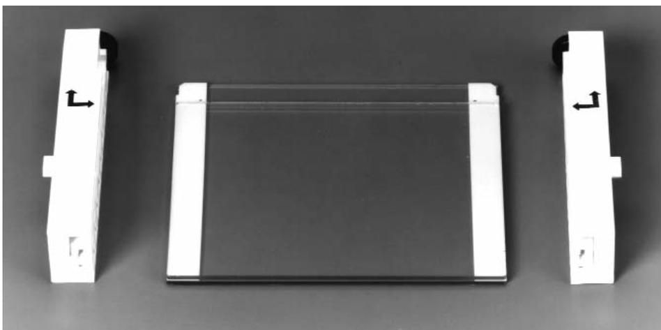
Fig. 4.10. Positioning glass plates, spacers, and clamps.
