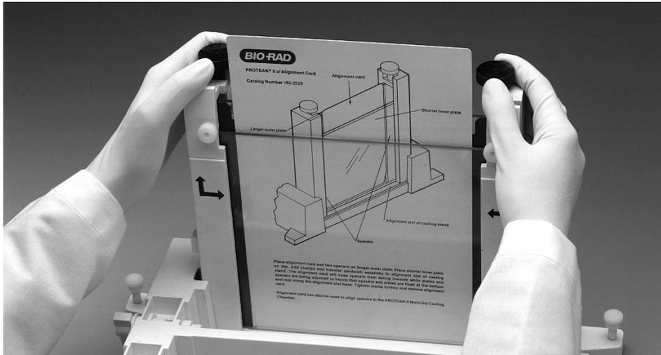
**Fig. 4.26. Aligning spacers in the sandwich assembly.**
