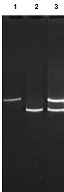
**Fig. 4.15. Constant denaturing gel. Amplified mutant and wild-type alleles of exon 8 from the p53 gene.** Separation by CDGE run at 130 V for 2.5 hours on a 10% acrylamide gel in 51% denaturant at 56 °C. Lane 1, mutant allele; lane 2, wild-type allele; lane 3, mutant and wild-type allele.
