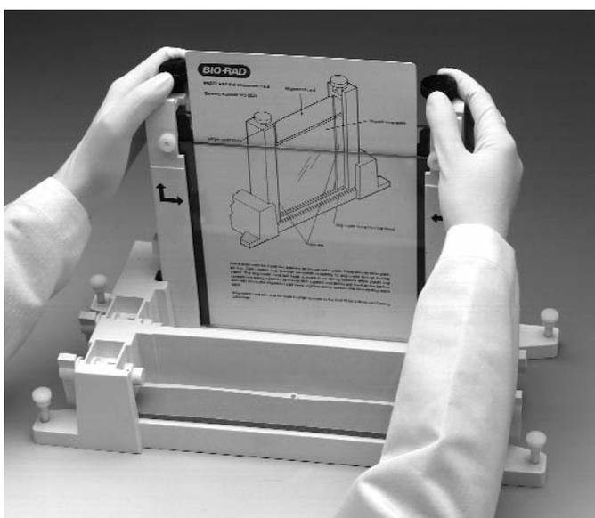
Fig. 7.4. Aligning spacers in the sandwich assembly.
