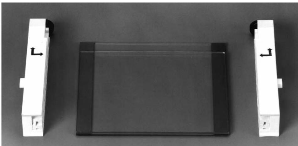
Fig. 5.2. Positioning glass plates, spacers, and clamps.
