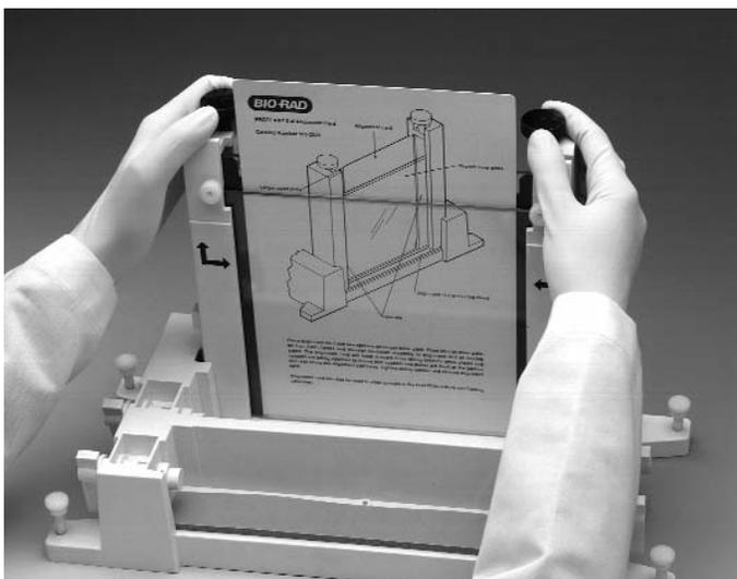
**Fig. 5.4. Aligning spacers in the sandwich assembly.**
