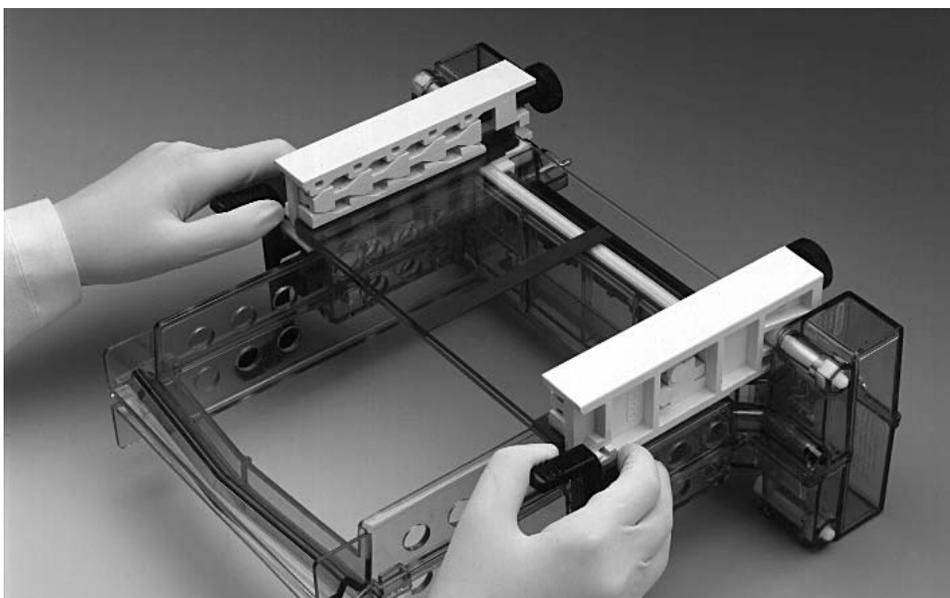
Fig. 8.2. Removing the sandwich assembly from the core.
