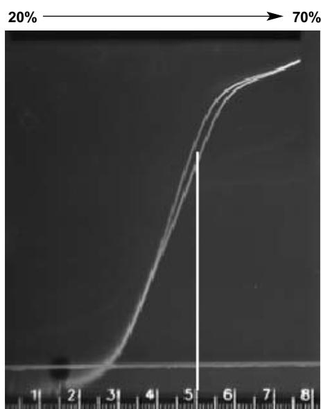
**Fig. 4.14. Example of perpendicular DGGE gel used for determining the optimum denaturant concentration used in a CDGE gel.** The distance along the gradient where the maximum split seen between samples is 5 cm. The denaturant concentration of the gradient at this distance is 51%. Therefore, the CDGE gel should use a denaturant concentration of 51%.
