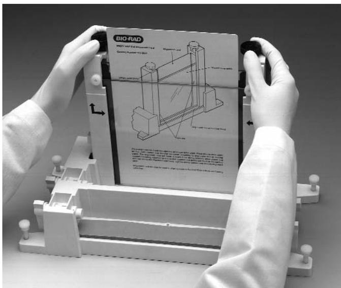
**Fig. 6.5. Aligning spacers in the sandwich assembly.**
