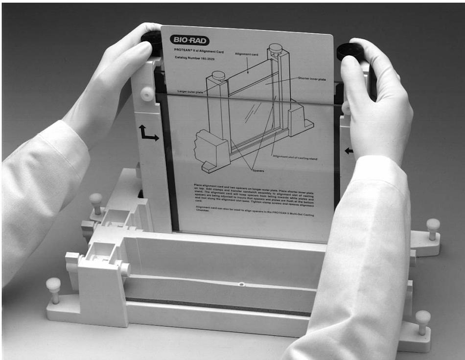
Fig. 4.7. Aligning spacers in the sandwich assembly.
