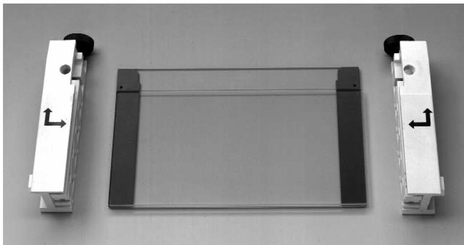
Fig. 4.5. Positioning glass plates, spacers, and clamps.
