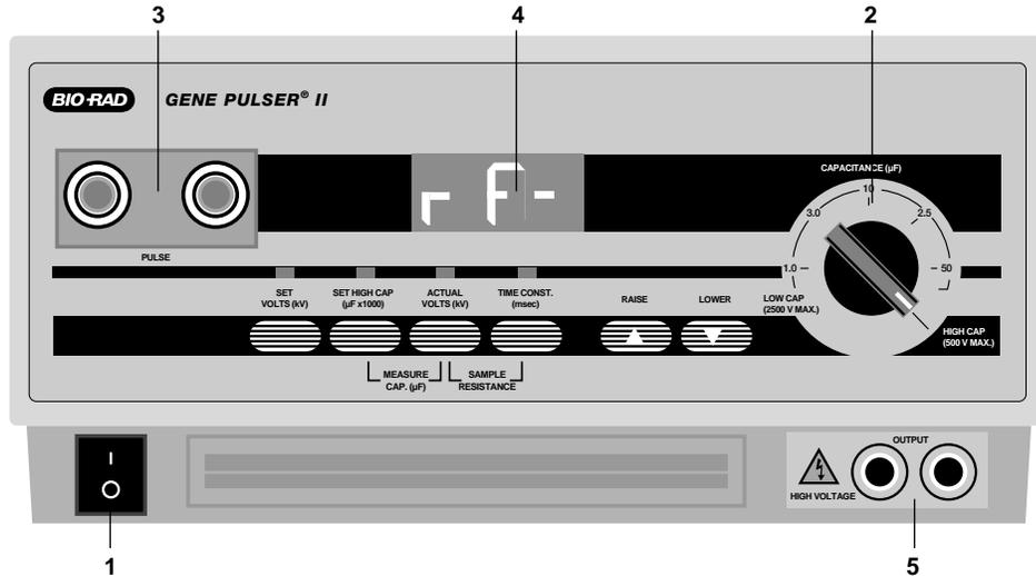
**Fig. 4. The control panel of the Gene Pulser II apparatus.** Front panel identification of switches and keypads for the Gene Pulser II unit. Note that the keypad(s) are active when the light(s) above them are illuminated.
