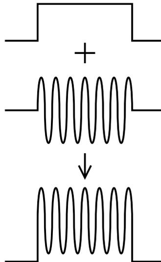
**Fig. 1. The FlexWave technology of the Gene Pulser II RF module delivers the unique combination of a pulse of radio-frequency (RF) field and a DC pulse with the same pulse width for improved transformation.**
