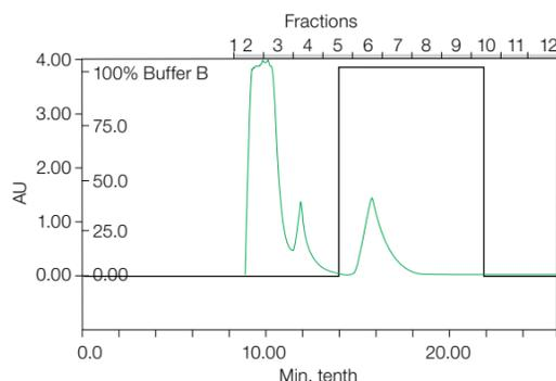
**Fig. 3. Purification of a 45 kD histidine-tagged protein on a Nuvia IMAC Column.** *E. coli* extract (2 ml) was loaded on a 0.46 x 5 cm column pre-equilibrated with 50 mM Na<sub>3</sub>PO<sub>4</sub>, 10 mM imidazole, and 300 mM NaCl, pH 7.5 (buffer A). The target protein was eluted with 10 CV 50 mM Na<sub>3</sub>PO<sub>4</sub>, 125 mM imidazole, 300 mM NaCl, pH 7.5 (buffer B). Column chromatography was monitored at OD 280. A<sub>280</sub> (—); %B (---). AU, absorbance units.
