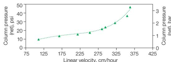
**Fig. 2. Pressure/flow performance of Nuvia IMAC Resin.** Uncharged Nuvia IMAC Resin slurry prepared in water was packed into a 20 x 20 cm column by axial compression using a compression factor of 1.2. The column pressure remained below 2 bar at a linear velocity of 300 cm/hr.
