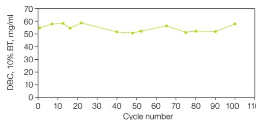
**Fig. 6. Reusability of Nuvia IMAC Resin.** A 45 kD histidine-tagged protein was loaded onto a 0.5 x 5.1 cm column packed with Nuvia IMAC with a compression factor of 1.25. The column was run at 300 cm/hr. The binding buffer was 50 mM sodium phosphate, 5 mM imidazole, and 300 mM NaCl (pH 7.5) and the elution buffer contained 250 mM imidazole. Solutions for column regeneration are listed in Table 1.
