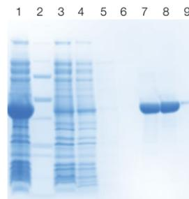
**Fig. 4. Analysis of column fractions from the purification of a 45 kD histidine-tagged protein on a Nuvia IMAC Column.** Fractions collected from the chromatography run shown in Figure 3 were analyzed by SDS-PAGE. Equal amounts (5 µl) were loaded onto the gel. Lane 1, *E. coli* lysate; lane 2, Precision Plus Protein™ Unstained Standards; lanes 3–9, fractions 3–9.
