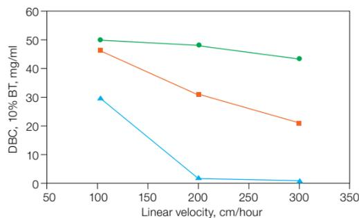
**Fig. 1. DBC vs. flow velocity of Nuvia IMAC Resin.** Comparison of DBCs between Nuvia IMAC (●), agarose IMAC resin A (■), and agarose IMAC resin B (▲). The resins were packed into 1 ml columns (0.5 x 5 cm). A 45 kD histidine-tagged protein (1.2 mg/ml) in 50 mM sodium phosphate, 5 mM imidazole, 300 mM NaCl (pH 7.5) was loaded onto each column until 10% breakthrough (BT) was observed.
