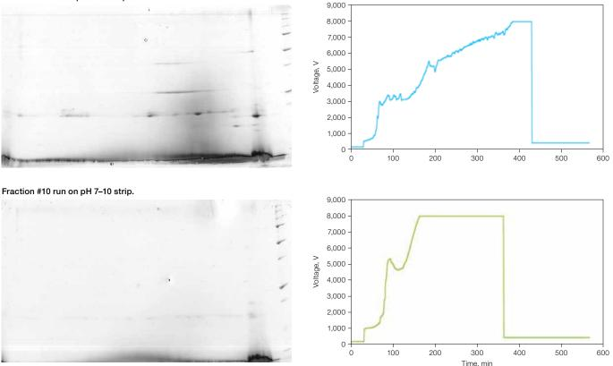
Fig. 1. 2-D gel images and voltage profiles of MicroRotofor cell focused in one run on the PROTEAN i12 IEF cell. All of the second-dimension gels were run on 8–16% Criterion Tris-HCl gels.
