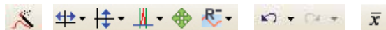
Fig. 8. Quick navigation to processing controls. From left to right: 3-point auto processing; individual processing keys for manual or automated X and Y alignment, spike removal, manual sensorgram movement, and referencing; undo and redo commands; report point generation commands.
