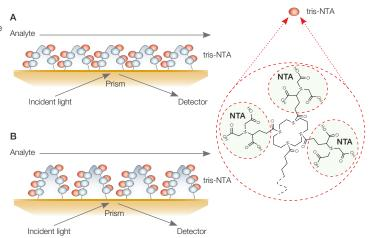
**ProteOn HTG and HTE sensor chips. A**, Alginate coating modified with compact-density tris-NTA on the HTG sensor chip; **B**, Alginate coating modified with high-density tris-NTA on the HTE sensor chip.
