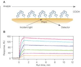
**ProteOn GLC sensor chip. A**, The thin alginate coating on the GLC sensor chip is responsible for creating a compact capacity surface. **B**, Sensorgrams of the cytokine IL-2 and an anti–IL-2 antibody interaction using the GLC sensor chip. The IL-2 Ab was immobilized to approximately 2,000 RU, and IL-2 was injected in a twofold dilution series ranging from 80 nM to 2.5 nM. The nearly planar surface of the GLC sensor chip allows for high-quality kinetic analysis.
