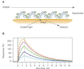
**ProteOn NLC sensor chip. A**, The NeutrAvidin-modified alginate coating on the NLC sensor chip. **B**, Sensorgrams of the interaction between an antibody Fab fragment and biotinylated MHC I/Tyr antigen using the NLC sensor chip. MHC I was captured to approximately 800 RU, and the Fab was injected in a twofold dilution series ranging from 500 nM to 31 nM.
