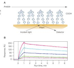
**ProteOn GLM sensor chip. A**, The extended alginate coating on the GLM sensor chip responsible for creating a medium-capacity surface. **B**, Sensorgrams of a TEM1  $\beta$ -lactamase mutant interacting with the  $\beta$ -lactamase inhibitor protein (BLIP) using the GLM sensor chip. TEM1 was immobilized to approximately 1,500 RU, and BLIP was injected in a twofold dilution series ranging from 600 nM to 38 nM.
