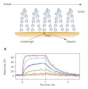
**ProteOn GLH sensor chip. A**, The dense alginate coating on the GLH sensor chip responsible for creating a high surface capacity. **B**, Sensorgrams of the interaction between carbonic anhydrase II (30 kD) and the inhibitor 4-carboxybenzenesulfonamide (CBS) (201 dalton) using the GLH sensor chip. Carbonic anhydrase II was immobilized to approximately 24,000 RU, and CBS was injected in a threefold dilution series ranging from 20  $\mu$ M to 0.082  $\mu$ M.
