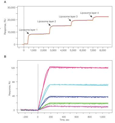
**ProteOn LCP sensor chip. A**, The planar NeutrAvidin surface and the LCP capturing reagent kit allow stable capturing of several POPC liposome layers. **B**, Detailed kinetic analysis of the interaction between FITC-labeled DSPC liposomes captured on the LCP sensor chip and an anti-FITC antibody. FITC-labeled DSPC liposomes were captured to approximately 330 RU, and the anti-FITC antibody was injected in a twofold dilution series ranging from 10 nM to 0.63 nM.
