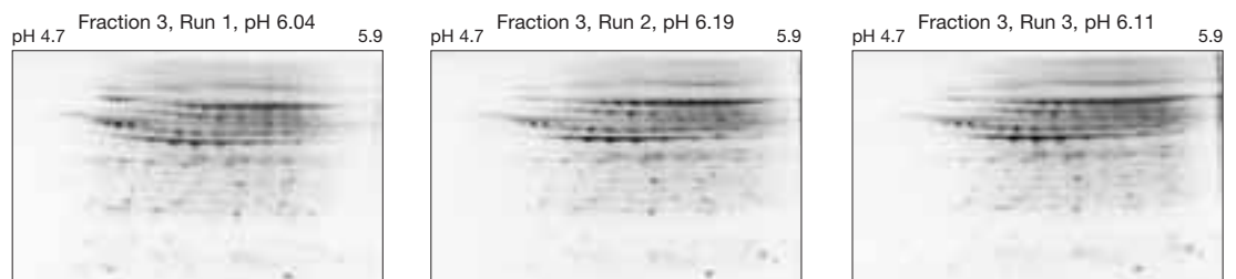
Fig. 3. Reproducibility of fractionation. 2-D separations of fraction 3 from three different MicroRotor runs are shown. First-dimension IEF was performed on micro-range (pH 4.7–5.9) IPG strips. The correlation coefficient of the three gels was 0.7.
