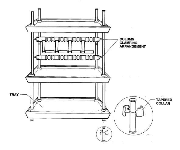
As you follow the procedure below, keep in mind that the illustration above is only an example. Alternative rack arrangements include mounting the column clamping arrangement on the side of the rack, mounting the column clamping arrangement to hold all columns outside the rack or short and/or heavy columns inside the rack, and setting up the rack to use only two trays.
