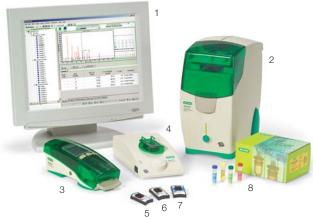
Experion automated electrophoresis system components.
