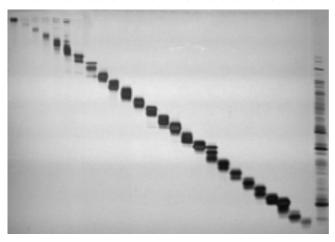
**Culture filtrates can be divided into narrow, sharply defined fractions on the whole gel eluter.** Culture filtrates (5 mg) were separated in a 10–20% SDS-PAGE gel, and the gel was electroeluted at 40 V for 20 min on the whole gel eluter. The fractions were analyzed on a 10–20% SDS-PAGE gel, and proteins were visualized by silver staining. Lane F, filtrate; lanes 1–26, fractions 1–26 off the eluter. No proteins were detected in lanes 27–30.
