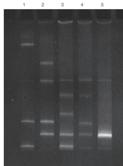
**Fig. 2. CDGE separation of  $\beta$ -thalassemia samples run on the DCode system.** Lane 1, compound mutant sample IVS1-1 + IVS1-6; lane 2, mutant sample IVS1-1; lane 3, mutant sample IVS1-6; lane 4, mutant sample IVS1-110; lane 5, wild-type DNA.
