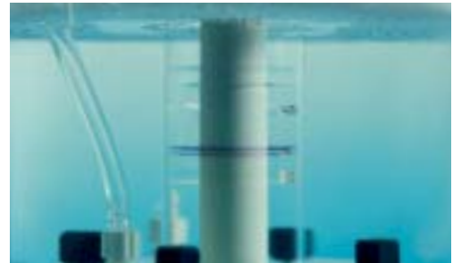
Phycocyanin subunits are visible as individual bands during separation on the Model 491 prep cell.
