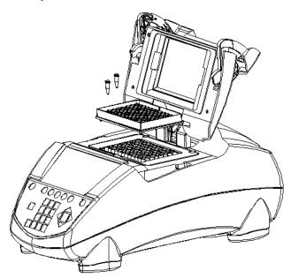
The MyCycler Sample Loading Tray is compatible with individual 0.2 ml thin wall tubes with domed caps (such as Bio-Rad 0.2 ml Thin-Wall Tubes, catalog number 223-9473). Once correctly positioned in the MyCycler instrument, the Sample Loading Tray can be left in the reaction block at all times. The multifunctional tray can also be used to transport PCR tubes between the workbench and the reaction block, or stacked upon an empty tray to serve as a post-PCR storage system for 0.2 ml tubes.
