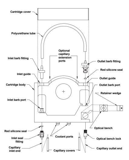
Fig. 1. BioFocus cartridge assembly diagram.
