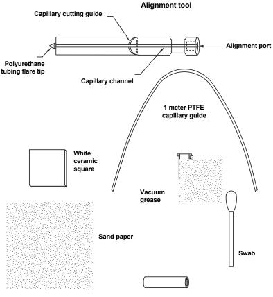
Inlet seal installation tool
