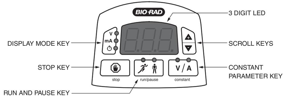
Fig. 3. Front Panel.
