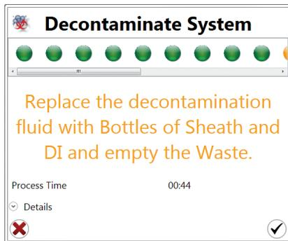
Fig. 135. Decontamination window prompting to replace fluidics.
