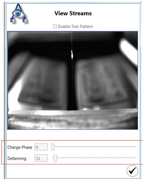
Fig. 38. View Streams window with charge phase and defanning slider bars highlighted.
