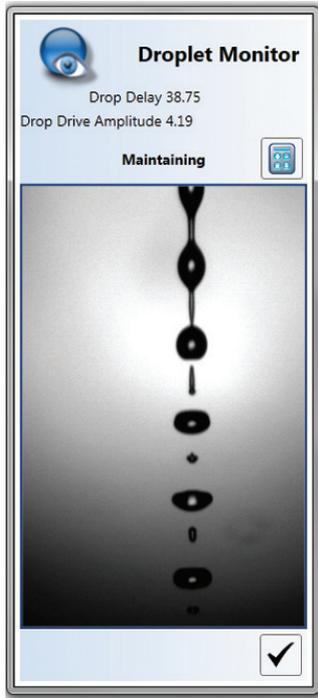
Fig. 37. Droplet Monitor window.
