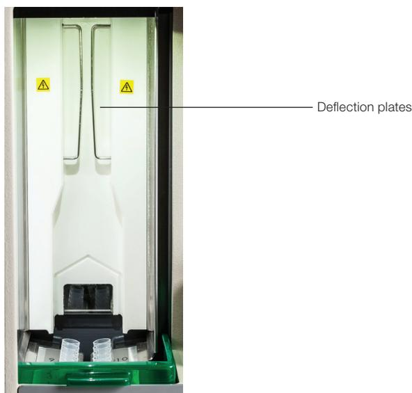
Fig. 9. Sort collection chamber and deflection plates.
