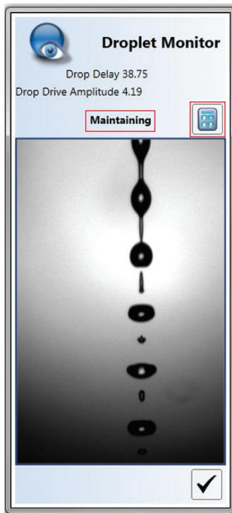
Fig. 41. Droplet Monitor window with status and recalculate button highlighted.
