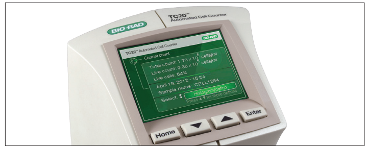
Fig. 3. Current count screen showing total cell count, live cell count, and percentage of live cells; cell viability is measured via trypan blue exclusion.
