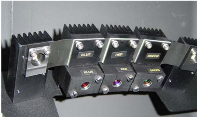
3. Match the module label with the same color label on the Epi lights bracket assembly.
