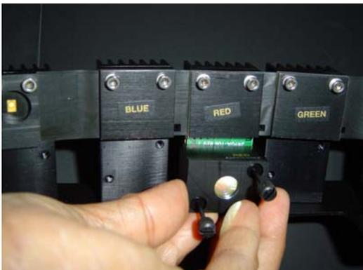
4. Position the module, contact tab up, against the bracket assembly so that the guide tabs are on the sides of the heat sink and the module cannot move sideways. Make sure the screws extend as shown in the picture and the module is flat against the heat sink.
