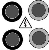
Insert power leads into one of the output terminals located on the front of the power supply (shown to the left). Note that the ⚠ symbol indicates high voltages and that the power leads must be inserted perpendicular to the curve of the case (see below).
