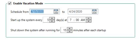
6. Specify how many minutes after startup should the system shut down.
