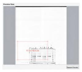
The densitometer scans the sample. As the scan progresses, Image Lab displays the scan in a scan area box outlined in red.
