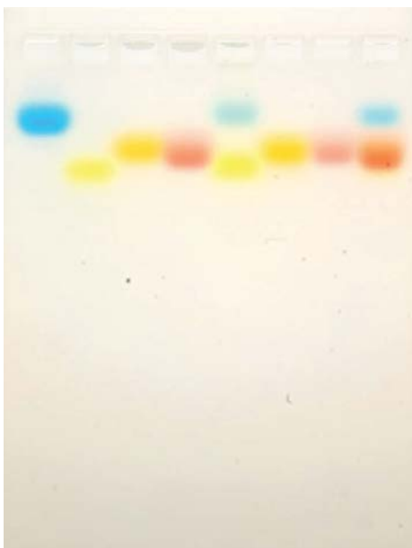
Fig. 2. Electrophoretic separation of standard dyes and color coatings extracted from standard U.S.-manufactured candies.
