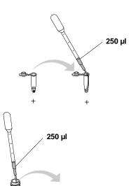
5. Using a well rinsed pipette, transfer 250 µl of binding buffer to the "+" supernatant. Place the tube in the refrigerator until the next laboratory period.
