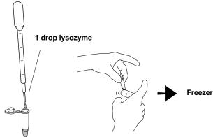
5. Place the microtube in the freezer until the next laboratory period. The freezing causes the bacteria to rupture completely.
