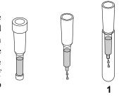
2. Using a new pipette, carefully and gently load 250 μl of the "+" supernatant onto the top of the column. Hold the pipette tip against the side of the column wall, just above the upper surface of the matrix and let the supernatant drip down the side of the column wall. Examine the column using a UV light. Note your observations. After it stops dripping transfer the column to collection tube 2.
