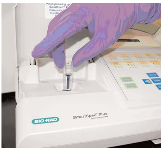
Fig. 5. Proper placement of a cuvette in the SmartSpec Plus.
