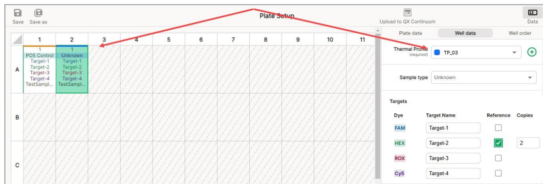
Fig. 2: Thermal profile assigned to well A2
