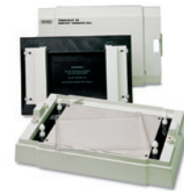
Semi-Dry Transfer Cells
