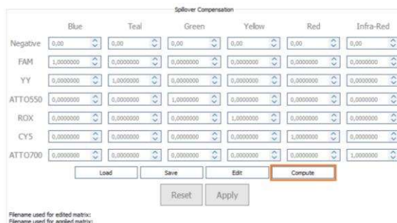
Figure 34: Compute button in the Spillover Compensation tab to generate a compensation matrix for a 6-plex assay.
