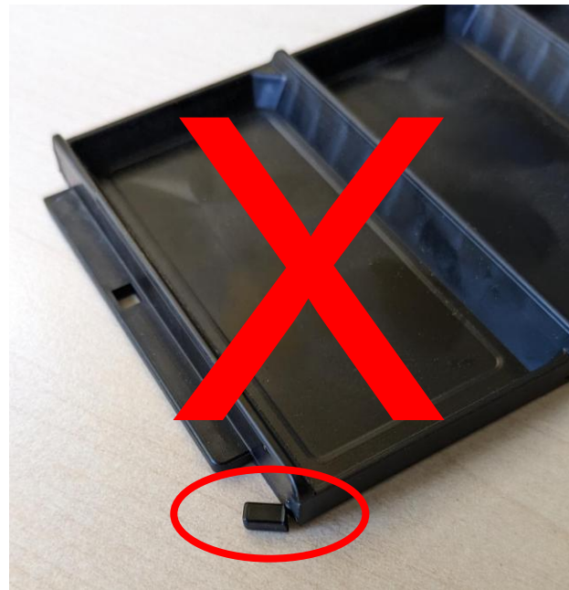
Figure 42 : Damaged Chip plate with broken pin
