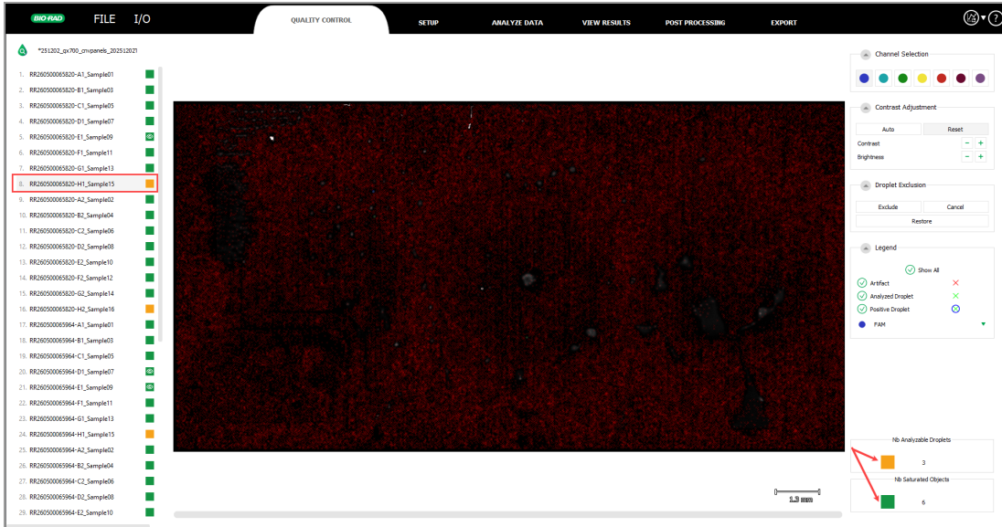
Fig. 3: Example of a droplet image in a chamber with a yellow flag
