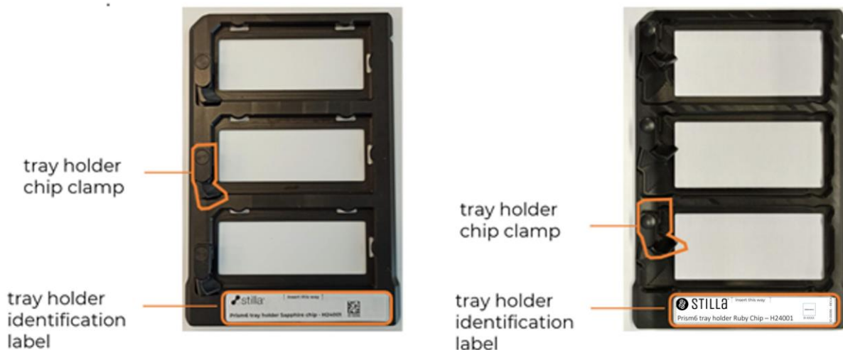
Figure 5: Prism6 tray holder Sapphire Chip H24002 (left) & Prism6 tray holder Ruby Chip H24001 (right)
