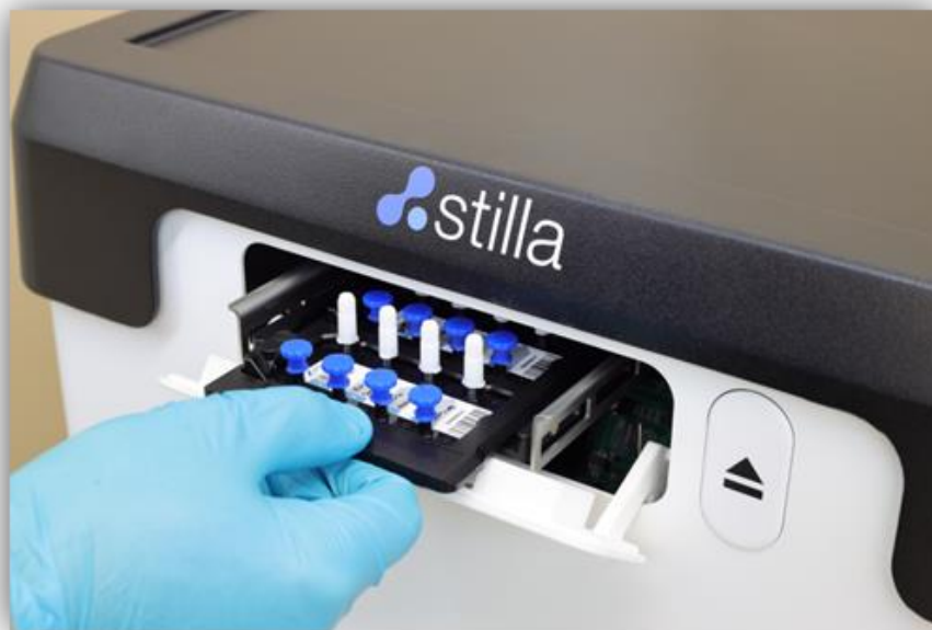
Figure 4: Fully ejected position of the movable tray. In this position, the moveable tray is ready to be loaded with the tray holder for chip scanning.
