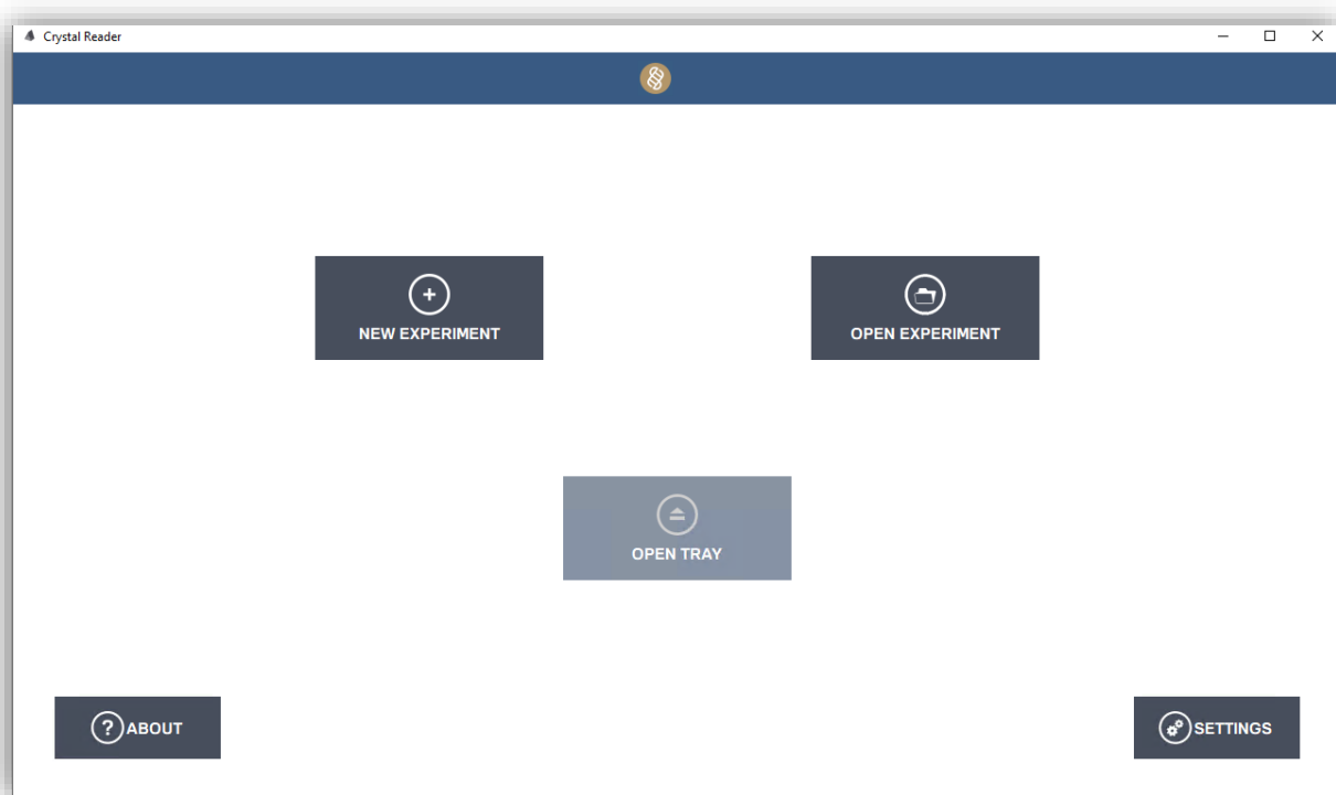
Figure 3: Crystal Reader software homepage with disabled “OPEN TRAY” button during Prism3 initialization or operation mode.
