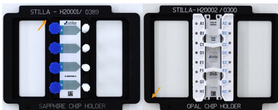
Figure 6: Positioning of the Sapphire Chip (left) and Ruby Chip (right) in the chip holder of the Prism3. The chip holder should be correctly oriented with error-proof cut-out upper-right hand corner for the Sapphire Chip and bottom-left for Ruby Chip (arrows).
