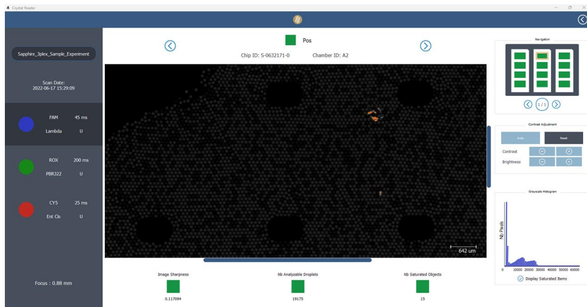
Figure 26: Overlay of the saturation map in the Blue detection channel in the Crystal Reader software (saturated pixels are displayed in orange color). In this case, they are dust particles.
