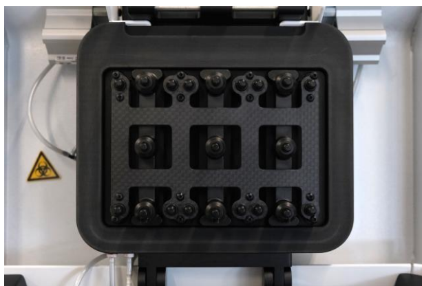
Figure 5: Magnetic Ruby Chip clip-on cushions can be easily clipped next to the existing pressure points.
