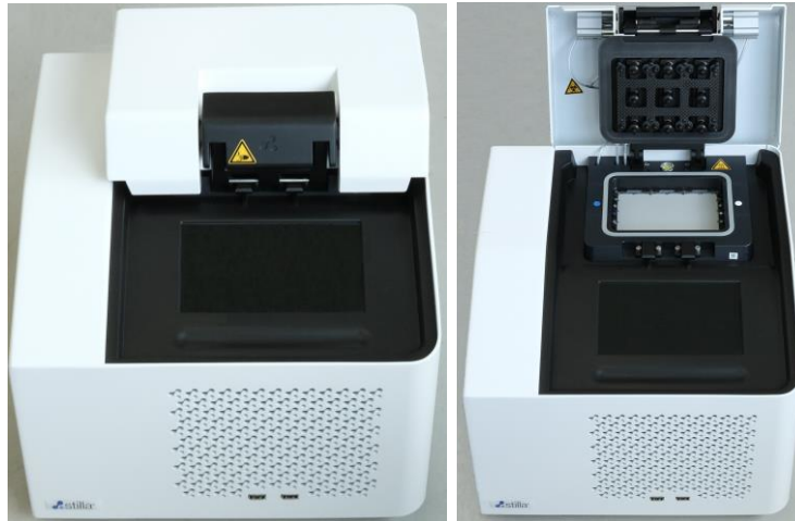
Figure 7: Opening/closing the lid of the Geode.
